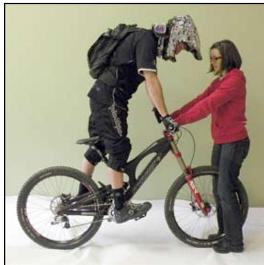
**4** Continue to stand still on the pedals and have your friend slide the indicator o-ring down against the wiper seal. This can be tricky, tell your friend to be quick!
