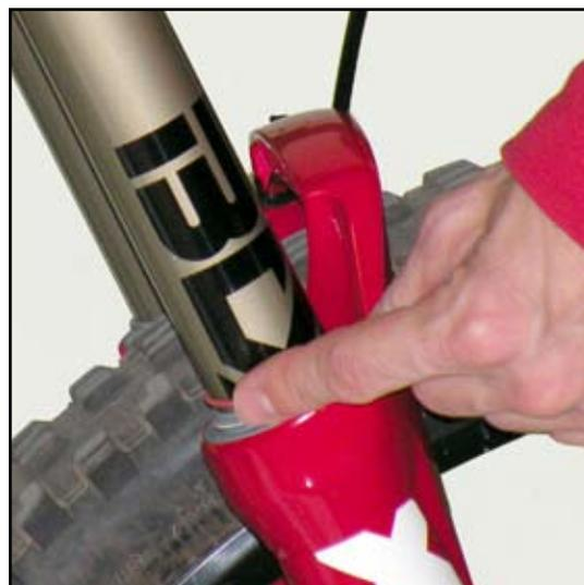
**5** Carefully step off the bike and compare the location of the travel indicator o-ring against the sag value gradients marked on the upper tube. This is your sag.
