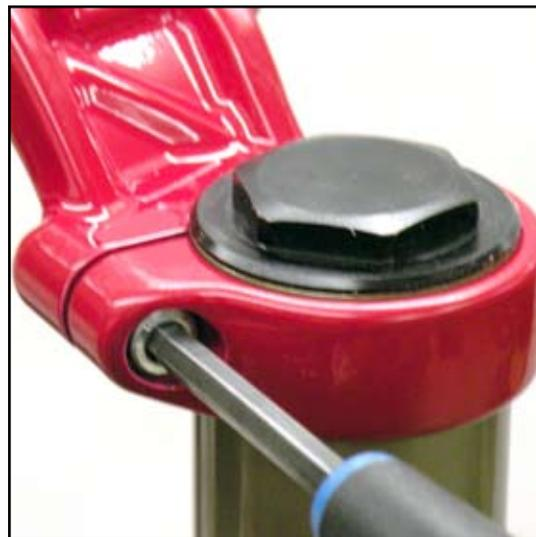
**2** Use a 24 mm socket wrench to loosen and remove the top cap located on the non-drive side fork leg. Be careful not to damage the top cap o-ring upon removal. If the top cap o-ring is damaged during removal, you must replace it with a new o-ring.
