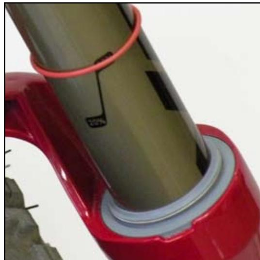
If you are unable to tune your fork to sag within the indicated range, you may need to change the fork's coil spring (coil spring tuning). Use the specific tuning information that follows to achieve proper sag.
