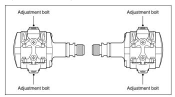
When the bolt is turned clockwise, the spring tension increases and the red part of the tension indicator becomes larger. When the bolt is turned all the way clockwise, it will suddenly become hard to turn. Do not turn the bolt beyond this point. When the bolt is turned counterclockwise, the spring tension decreases and the red part of the tension indicator becomes smaller. Once the red part of the tension indicator can no longer be seen, do not turn the bolt counterclockwise any further.
