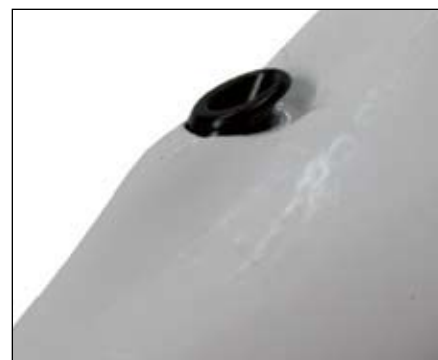
Figure 22. Down tube housing stop, several inches below the head tube
