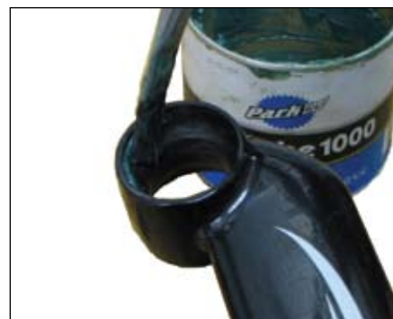
Figure 2. Applying grease to the socket of the seatmast cap (NOT '10 Madone 6 Series)
