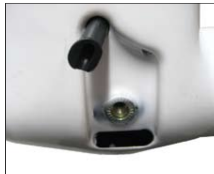
Figure 16. Bottom bracket inner-wire guide tube
