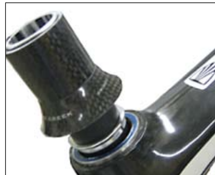
Figure 45. Sliding the shims and bearing cover onto the steerer
