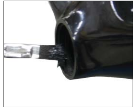
Figure 77. Greasing the bearing cups
