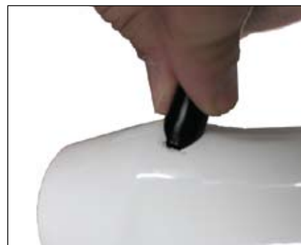
Figure 36. Engaging the threads of the "bolt" part of the housing stop with the "nut" inside the head tube
