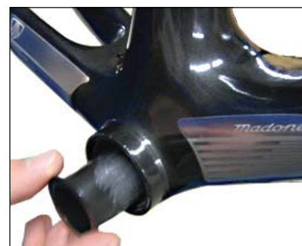
Figure 89. Inserting one half of the axle shield into frame
