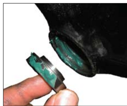
Figure 56. Grease on the frame and the non-drive side bearing (with the lip facing in)
