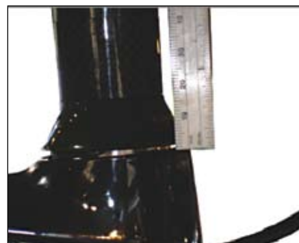
Figure 46. Measure the distance from the head tube to the bearing cover
