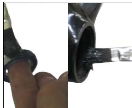
Figure 55. Greasing the bearing and the frame saddle
