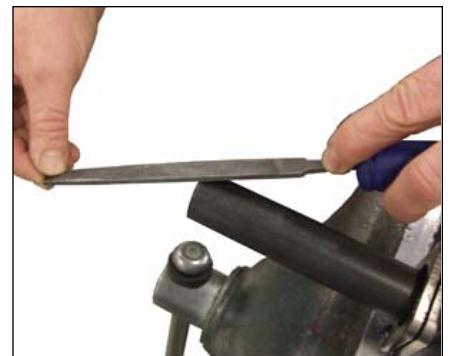
Figure 11. File away from the crown (NOT toward it)
