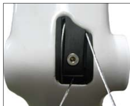
Figure 24. The inner-wire for the rear derailleur runs in the drive-side hole
