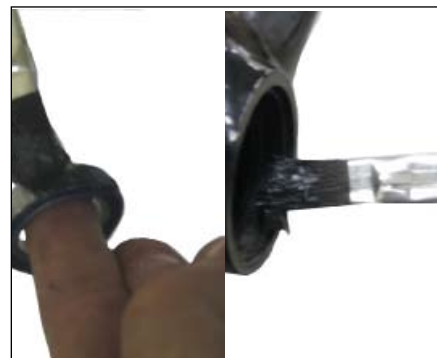
Figure 64. Greasing the bearing and the frame seat
