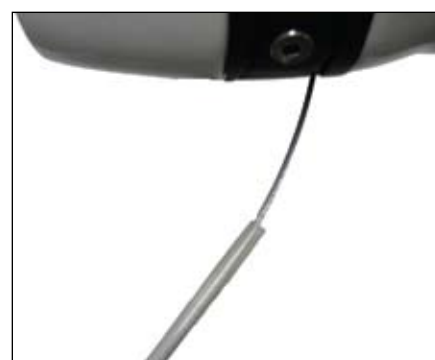
Figure 27. The inner-wire for the front derailleur runs in the drive-side hole
