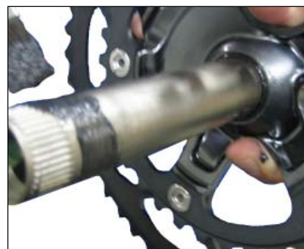
Figure 68. Greasing the axle
