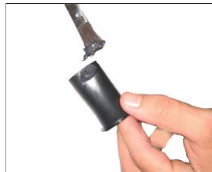
Figure 50. Applying grease to the axle shield
