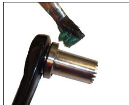
Figure 76. Greasing the bearings
