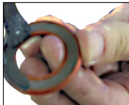
Figure 58. Greasing the bearing covers
