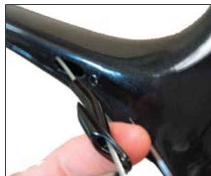
Figure 32. Sliding the frame ferrule up the brake inner-wire
