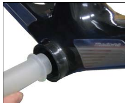
Figure 65. Pressing the bearing into the frame
