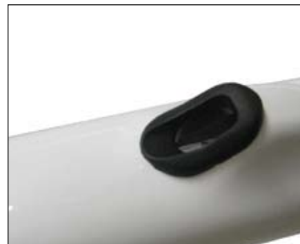
Figure 47. Hole through the chainstay for DuoTrap sensor
