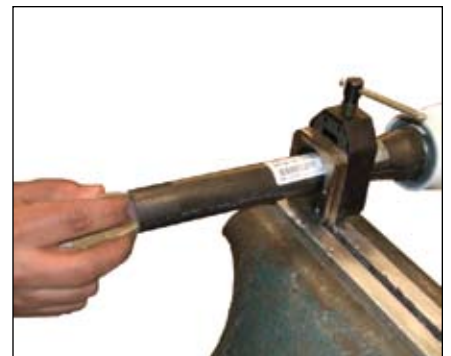
Figure 12. Smooth the inside of the steerer with fine-grit sandpaper
