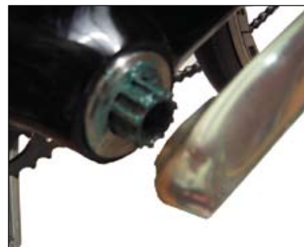
Figure 62. Metal bearing cover in place over the bearing
