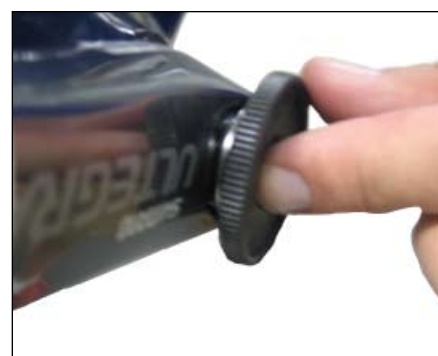
Figure 71. Pressing the crank arm onto the axle
