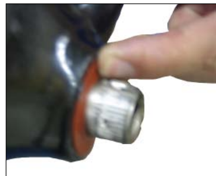
Figure 70. Pressing in the second bearing cover
