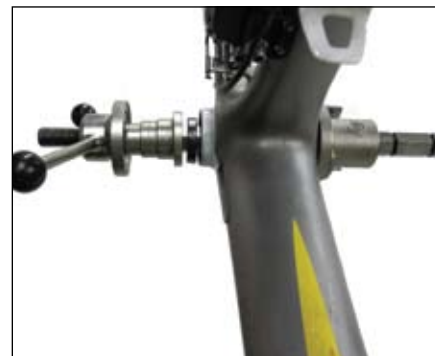
Figure 53. Using a headset press to install the bearings
