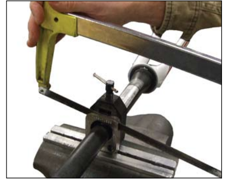
Figure 9. Use light pressure when cutting.
