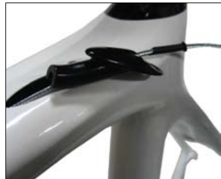
Figure 38. Attaching the housing stop with the fixing screw
