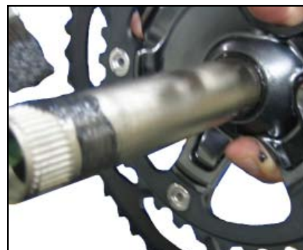
Figure 84. Greasing the axle
