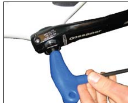
Figure 86. Pressing the crank arm onto the axle
