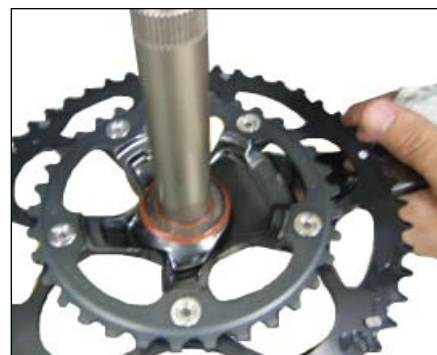
Figure 67. Sliding the bearing cover onto the axle
