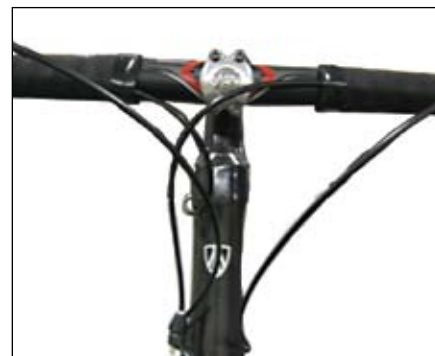
Figure 13. Inner-wire routing around the head tube
