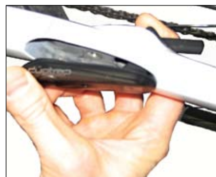
Figure 48. Sliding the speed cylinder of a DuoTrap sensor through the chainstay
