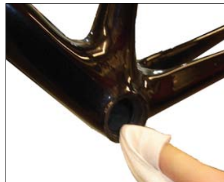
Figure 73. Cleaning bonding surfaces with an alcohol wipe
