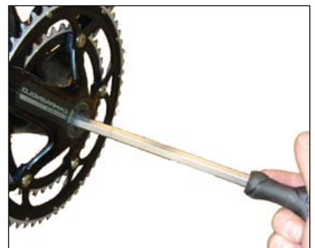
Figure 80. Tightening the axle bolt
