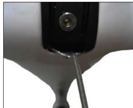
Figure 23. A J-bend spoke can grasp the inner-wire, and then you can pull the inner-wire through the guide
