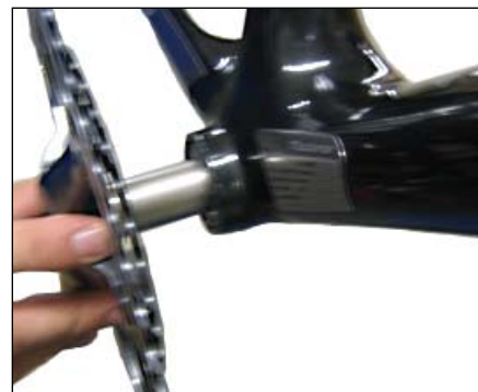
Figure 69. Sliding the axle through the bearings
