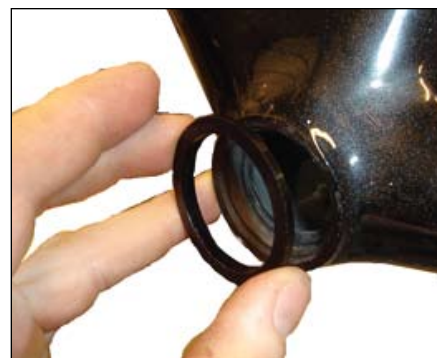
Figure 75. Inserting the bearing cups into the bottom bracket shell
