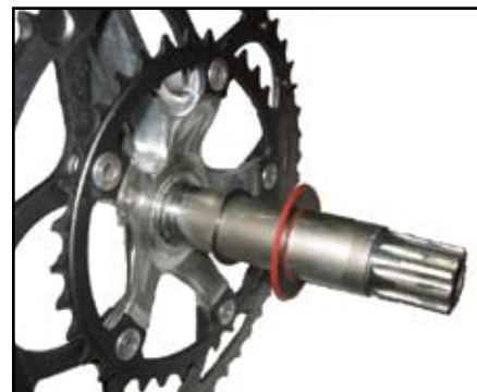
Figure 59. Sliding the wave washer and bearing cover onto the axle
