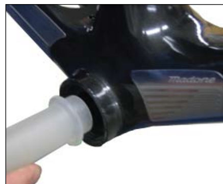
Figure 57. Pressing the bearing into the frame
