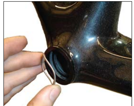
Figure 78. Inserting the Wave washer (after the washer) on the non-drive side
