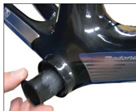
Figure 51. Inserting one half of the axle shield into frame
