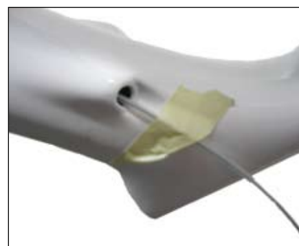
Figure 28. The inner-wire for the front derailleur runs in the drive-side hole
