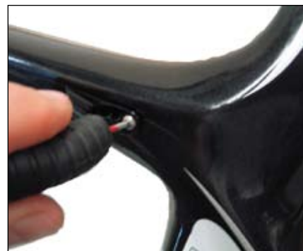
Figure 29. Removing the fixing screw for the rear housing stop
