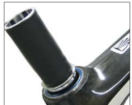
Figure 44. Slide the compression washer onto the steerer
