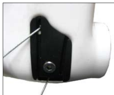
Figure 20. The inner-wire for the front derailleur runs in the non-drive-side hole
