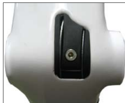
Figure 25. The inner-wire should lay in the groove of the guide
