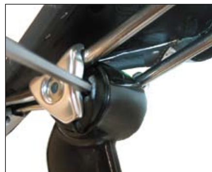
Figure 8. Prying the locking cones loose with a 4 mm allen wrench
