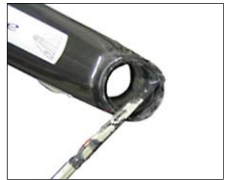
Figure 42. Greasing upper bearing saddle
