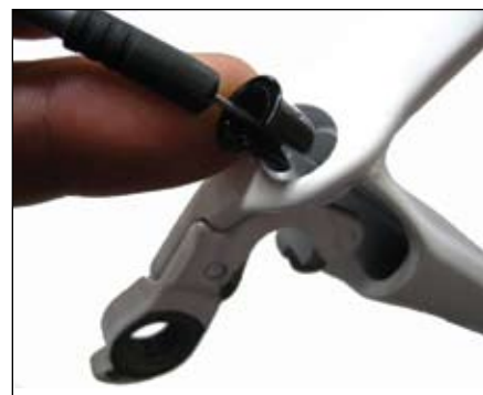
Figure 26. Housing stop and housing in the chainstay
