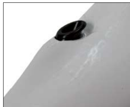
Figure 18. Down tube housing stop, several inches below the head tube
