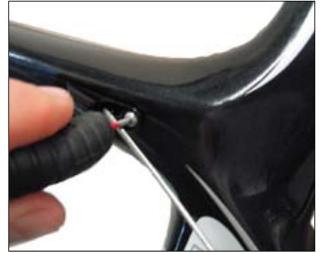
Figure 33. Attaching the housing stop with the fixing screw
