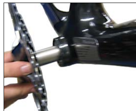
Figure 61. Sliding the axle through the bearings
