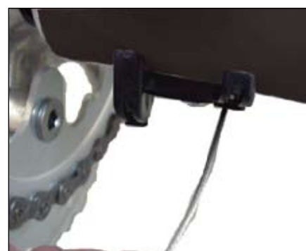
Figure 14. Front derailleur inner-wire on the rider's left of the bottom bracket inner-wire guide
