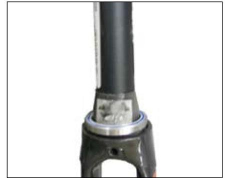
Figure 41. Lower bearing on fork crown
