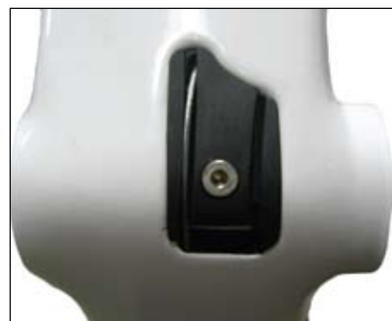
Figure 21. The inner-wire should lay in the groove of the guide
