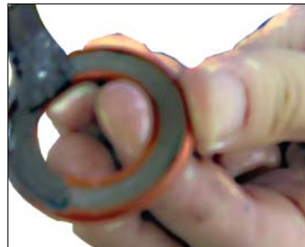
Figure 66. Greasing the bearing covers
