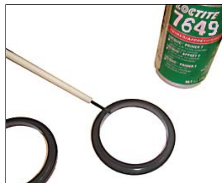
Figure 74. Applying Loctite primer to the outer step of the bearing cups
