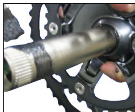
Figure 60. Greasing the axle
