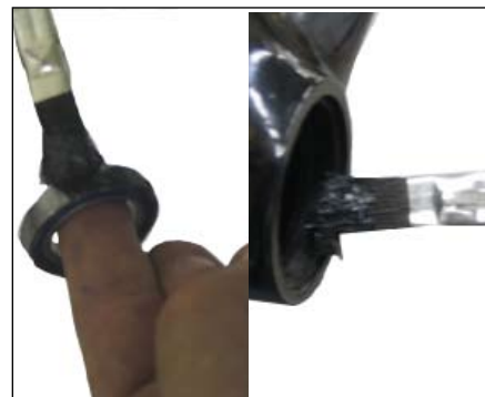
Figure 82. Greasing the bearing and the frame saddle
