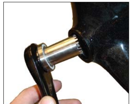
Figure 79. Inserting the non-drive side axle
