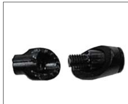
Figure 34. "Nut" (left) and "bolt" of head tube housing stop
