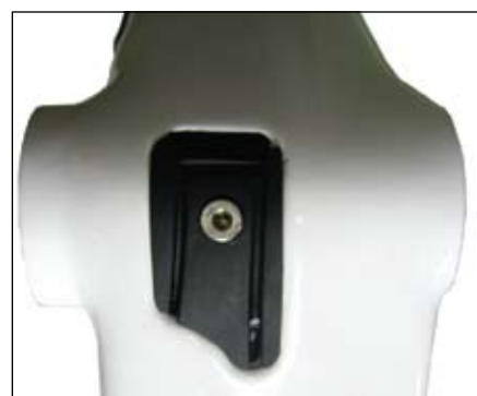
Figure 17. Bottom bracket inner-wire guide
