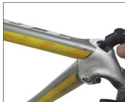
Figure 10. The electric cable for the rear derailleur passing through the dropout
