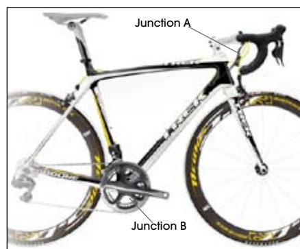
Figure 8. Madone with Di2 showing locations of junction boxes
