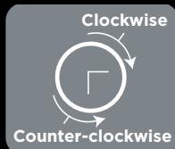
"Clockwise" and "counter-clockwise" apply to knob or lever control turning direction, which is relative to your facing the control straight on. This is consistently true for all FOX forks and rear shock products.
