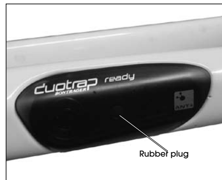
Figure 3. DuoTrap sensor installed on chainstay
