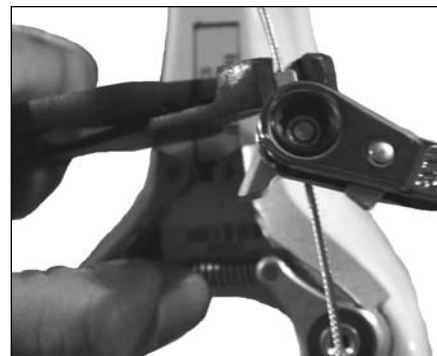
Figure 5. Holding the wedge while tightening the cable clamp nut
