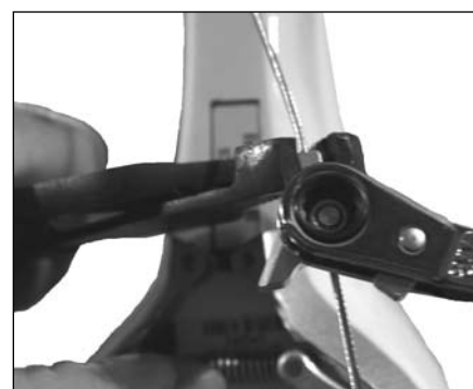
Figure 6. Hold the wedge while you tighten the clamp bolt
