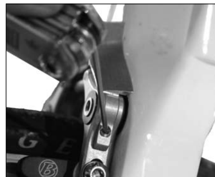
Figure 8. Adjusting screw for front brake (screw is accessible through cover)
