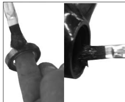
Figure 11. Greasing the bearing and the frame saddle
