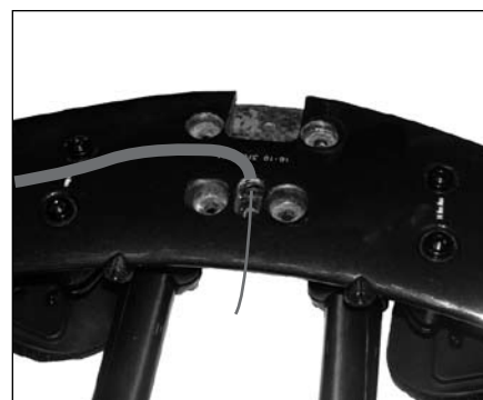
Figure 3. Housing (and cable) route through aerobar for low/near and medium/near stems
