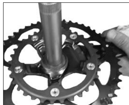
Figure 5. Sliding the bearing cover onto the axle
