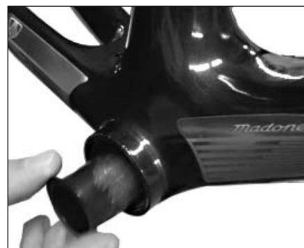
Figure 2. Inserting one half of the axle shield into frame
