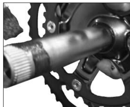
Figure 6. Greasing the axle
