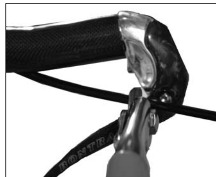
Figure 5. Setting the length and cutting the housing
