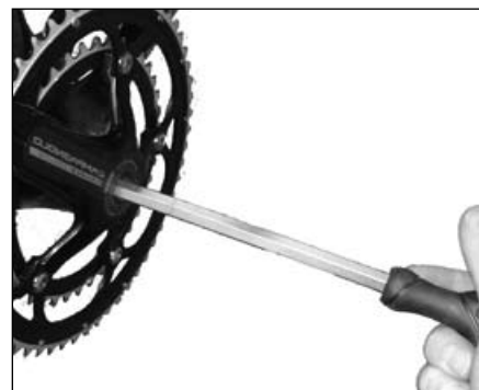
Figure 9. Tightening the axle bolt
