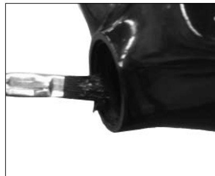
Figure 6. Greasing the bearing cups
