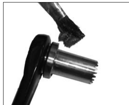
Figure 5. Greasing the bearings
