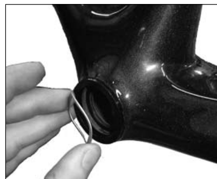
Figure 7. Inserting the Wave washer (after the washer) on the non-drive side
