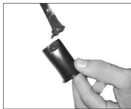
Figure 1. Applying grease to the axle shield
