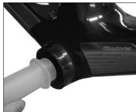
Figure 3. Pressing the bearing into the frame
