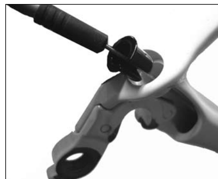
Figure 4. Rear derailleur cable passing through the dropout housing stop
