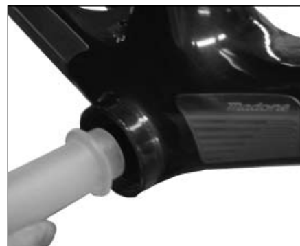
Figure 3. Pressing the bearing into the frame
