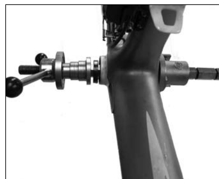
Figure 1. Using a headset press to install the bearings
