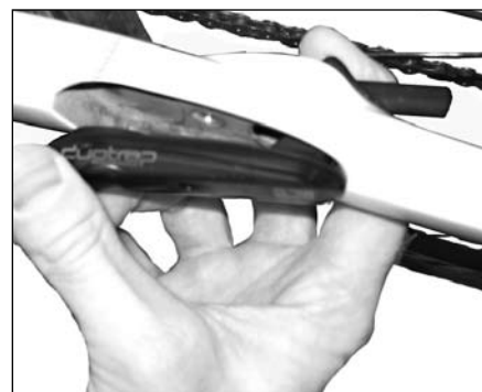
Figure 2. Sliding the speed cylinder of a DuoTrap sensor through the chainstay
