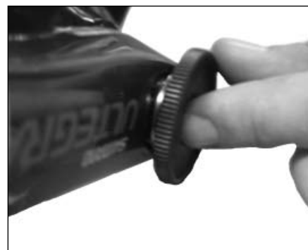
Figure 9. Pressing the crank arm onto the axle
