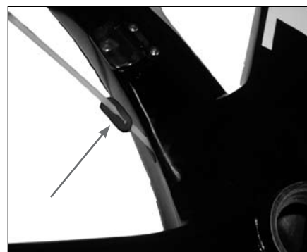
Figure 3. Seat tube grommet on cable liner to front derailleur
