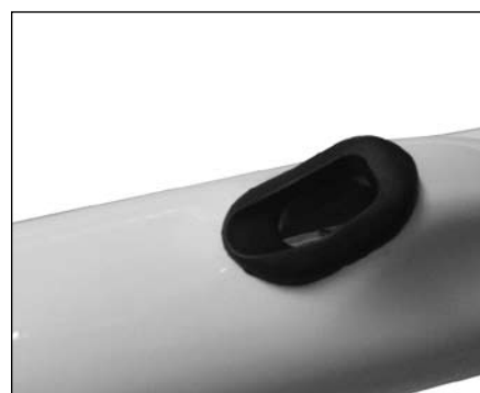
Figure 1. Hole through the chainstay for DuoTrap sensor
