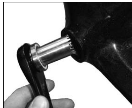
Figure 7. Sliding the axle through the bearings
