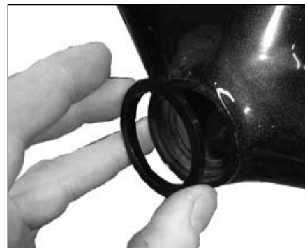
Figure 4. Inserting the bearing cups into the bottom bracket shell
