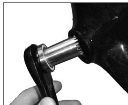
Figure 8. Inserting the non-drive side axle
