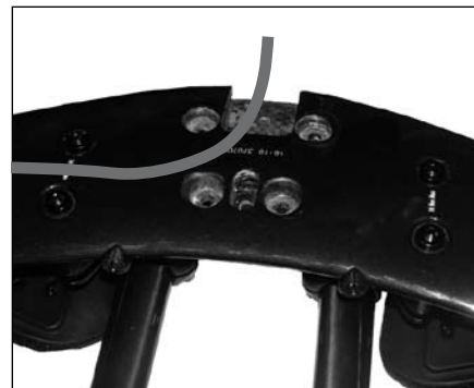
Figure 4. Housing route through aerobar for all stems except low/near and medium/near
