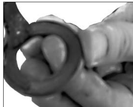
Figure 4. Greasing the bearing covers
