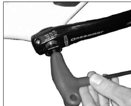
Figure 15. Pressing the crank arm onto the axle
