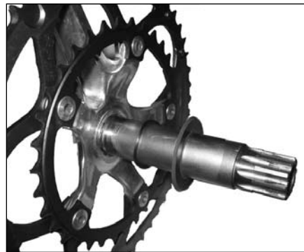
Figure 5. Sliding the wave washer and bearing cover onto the axle
