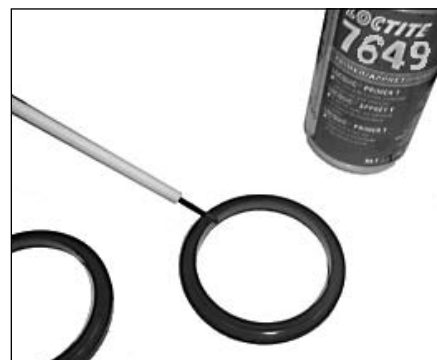
Figure 3. Applying LocTite primer to the outer step of the bearing cups
