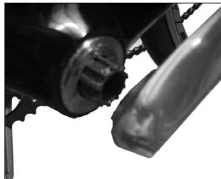
Figure 8. Metal bearing cover in place over the bearing
