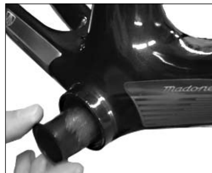
Figure 3. Inserting one half of the axle shield into frame
