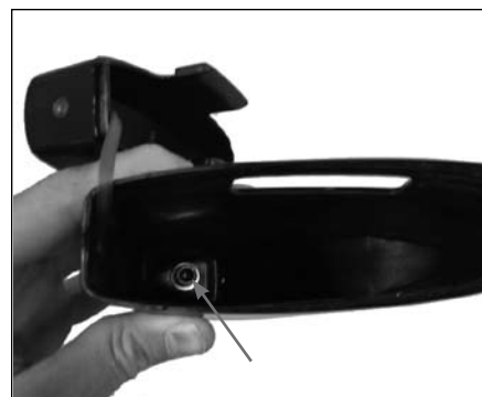
Figure 2. Clamp bolt in bottom of draft box
